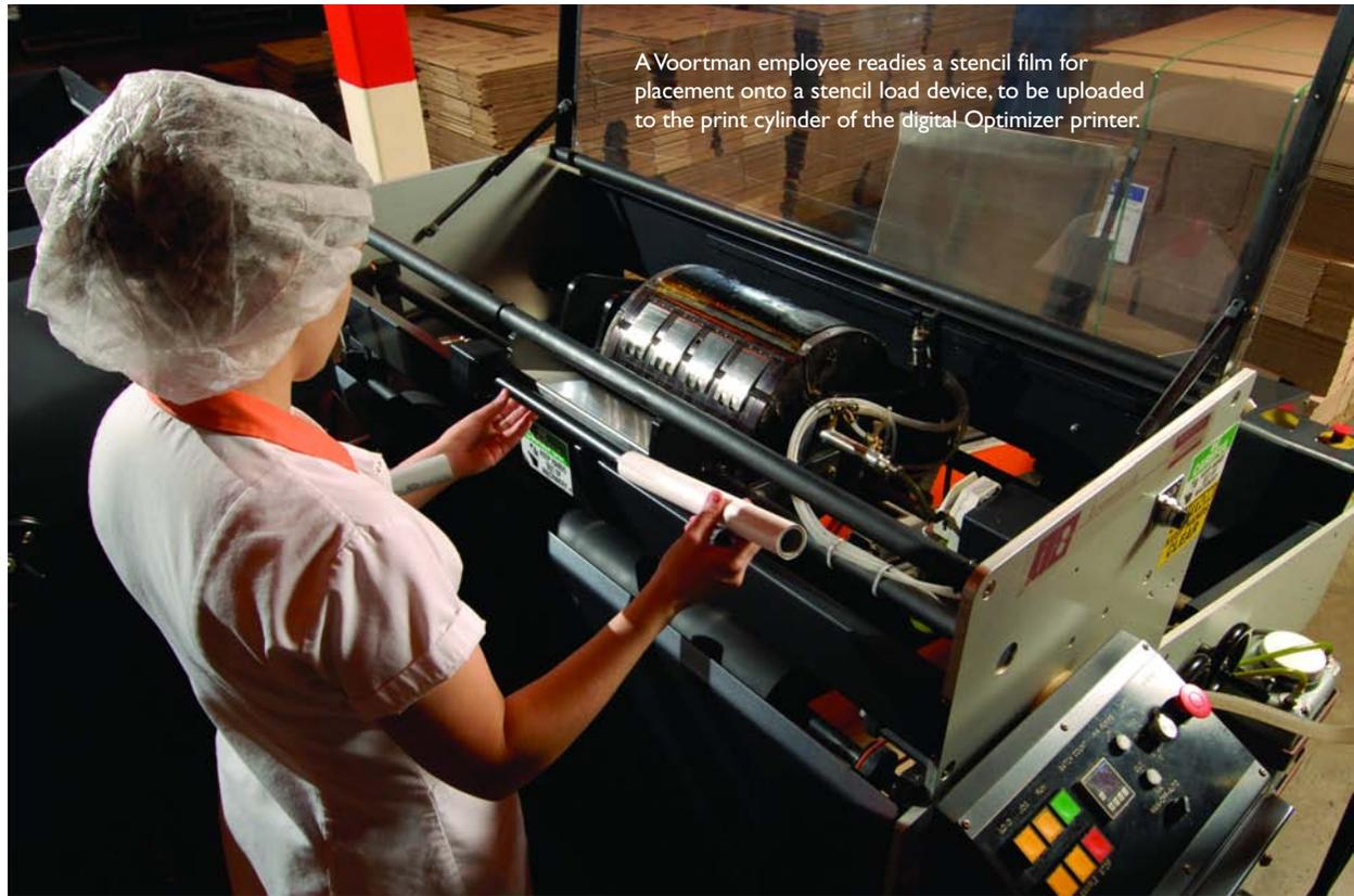
A Voortman employee readies a stencil film for placement onto a stencil load device, to be uploaded to the print cylinder of the digital Optimizer printer.
